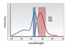
Variable bandwidth selection from 3 nm to 50 nm in 1 nm increments offers great versatility and is ideal for fluorophores with small Stokes shifts, broad excitation/emission bands, or for FRET and multiplexed assays where wavelength specificity is critical. Four holographic gratings are used to eliminate stray light and increase signal-to-background ratios, ensuring consistent performance for every read.
